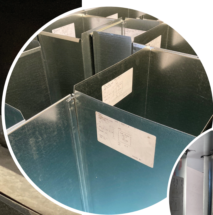
Ductwork made in C&S Cos.' Syracuse, New York, sheet metal shop. The industrial HVAC contractor added duct fabrication services in June 2023.
