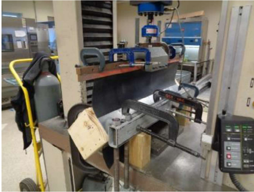
Photo No. 1 ANSI/SPRI Test RE-1 Test Set-up
