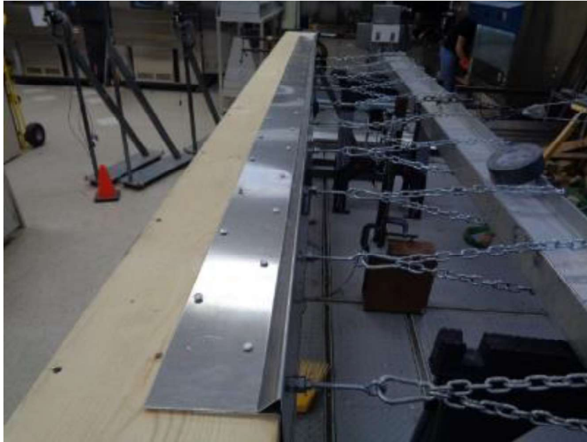
Photo No. 3 ANSI/SPRI Test RE-2, Test Setup
