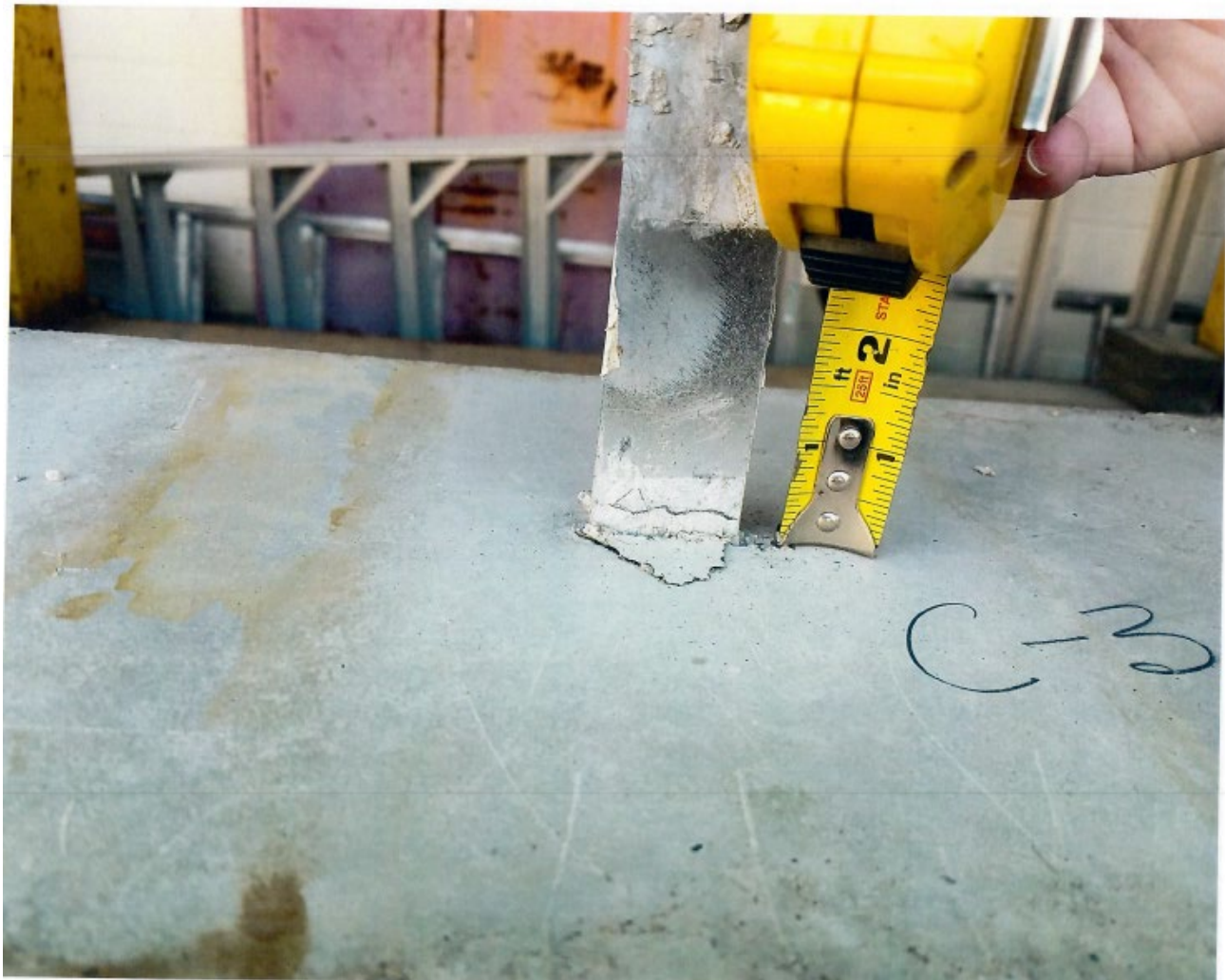
Figure 8 Sample Specimen C-3, Failure Mode for 16 Gage 1 ½ Inch Double Wide Coil Straps, Hanger Embedded 1 Inch From the Concrete Surface
