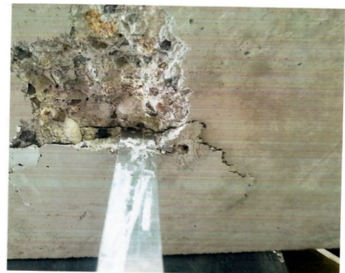
Figure 5 Sample Specimen Failure Mode for 16 Gage 1 Inch Wide Double Wide Coil Straps, Hanger Flush with Bottom of Concrete Surface
