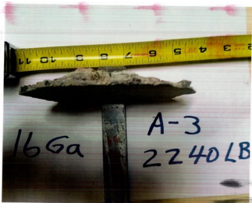
Figure 6 Sample Specimen A-3 Failure Mode for 16 Gage 1 Inch Wide Double Coil Straps, Hanger Flush with Bottom of Concrete Surface
