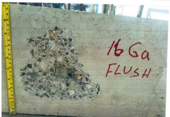
Figure 5 Sample Specimen Failure Mode for 16 Gage 1 Inch Wide Double Wide Coil Straps, Hanger Flush with Bottom of Concrete Surface
